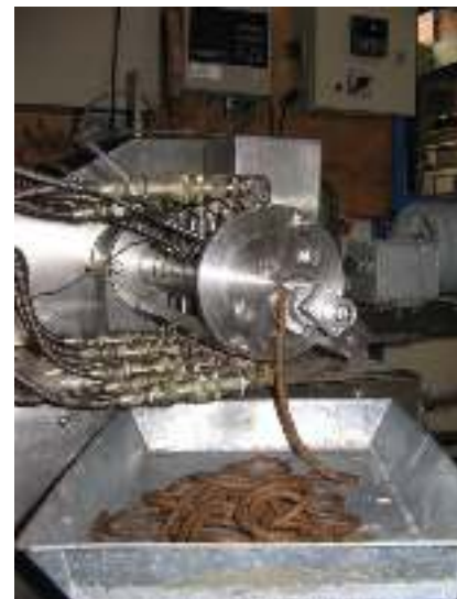
Photograph 7b. Calculation of the expansion index in a Wenger X-5 extruder
