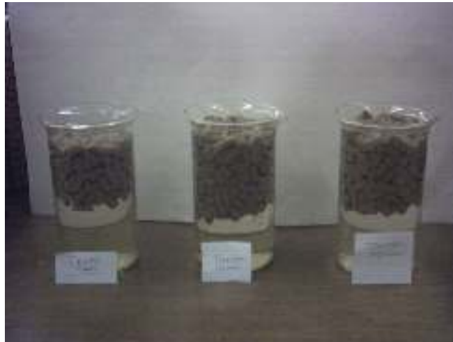
Photograph 6. Test for hydrostability of tilapia's feedstuffs using Plecostomus punctatus meal with other nutrients, example of use of die with orifice diameter of 2mm
